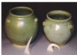
Some glazes look okay when underfired a little (on left), but create different effects when reaching their full temperature. (Sample Amaco glaze photos from Arts & Activities magazine, February 2015)
